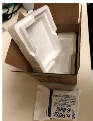
Place specimens upright in box, support with bubble-wrap to prevent shifting. Add frozen gel-pak, close styrofoam lid, place batch list between, tape box lid closed
