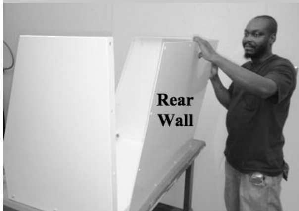
FIGURE 7. JOINING THE BACK TO THE BASE AND SIDES
