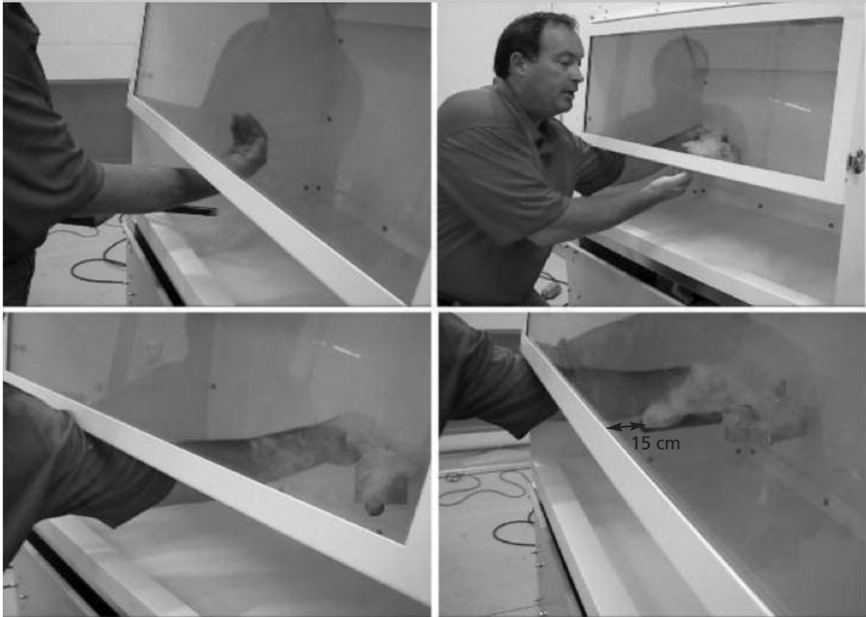
FIGURE 31. AIRFLOW SMOKE TEST – INTERNAL PERIMETER
