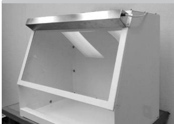
FIGURE 11. EXTERNAL LIGHT SOURCE
