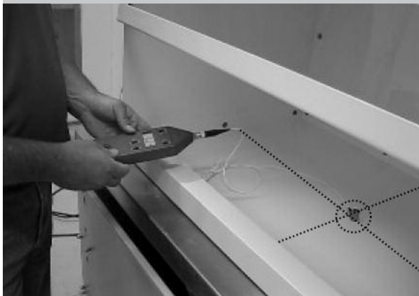
FIGURE 21. VIBRATION TEST – PLACING THE PROBE 1
